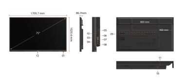
1. Smart Port USB<sup>™</sup> X 2 2. Camera 8. Audio Out 9. VESA® Wall Mount800 x 400mm
