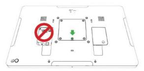
3 Plug Elo power-over-ethemet (POE) adaptor into recess, ensuring connector on bottom of adaptor lines up with connector on back of the I-Series 2.0.
