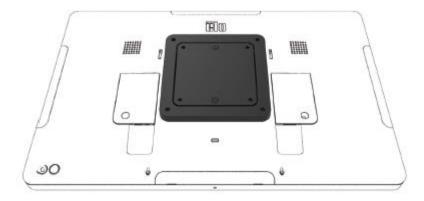
Attach VESA mounting bracket (not included) with screws long enough to pass through the adaptor and into the threaded holes of the I-Series 2.0 VESA mount. Elo recommends M4x16mm screws. Exact length of screws depends on thickness of VESA mount.
