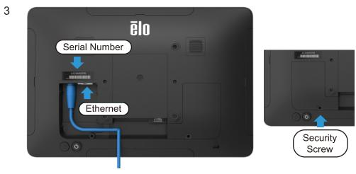
Connect an Ethernet cable now (or setup WiFi later). Once all cables are connected, reinstall the cable over and secure with included security screw.
